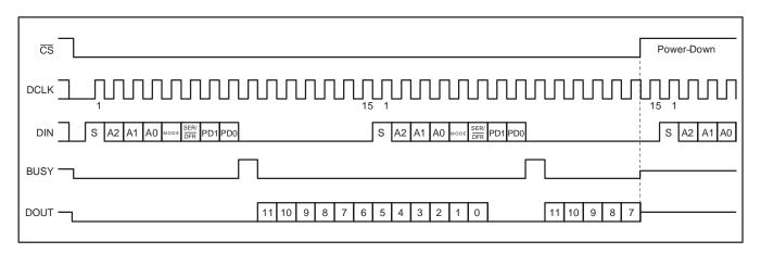
Figure 13. Maximum Conversion Rate, 15 Clocks-per-Conversion
