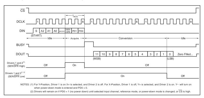
Figure 9. Conversion Timing, 24 Clocks-per-Conversion, 8-Bit Bus Interface.
