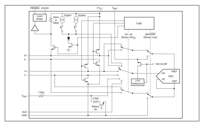
Figure 2. Simplified Diagram of Analog Input
