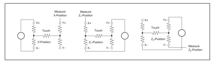
Figure 8. Pressure Measurement Block Diagrams
