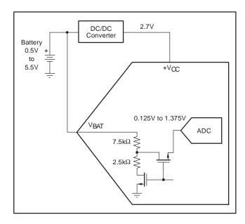
Figure 7. Battery Measurement Functional Block Diagram
