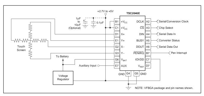
Figure 1. Basic Operation of the TSC2046E
