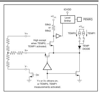
Figure 10. PENIRQ Functional Block Diagram
